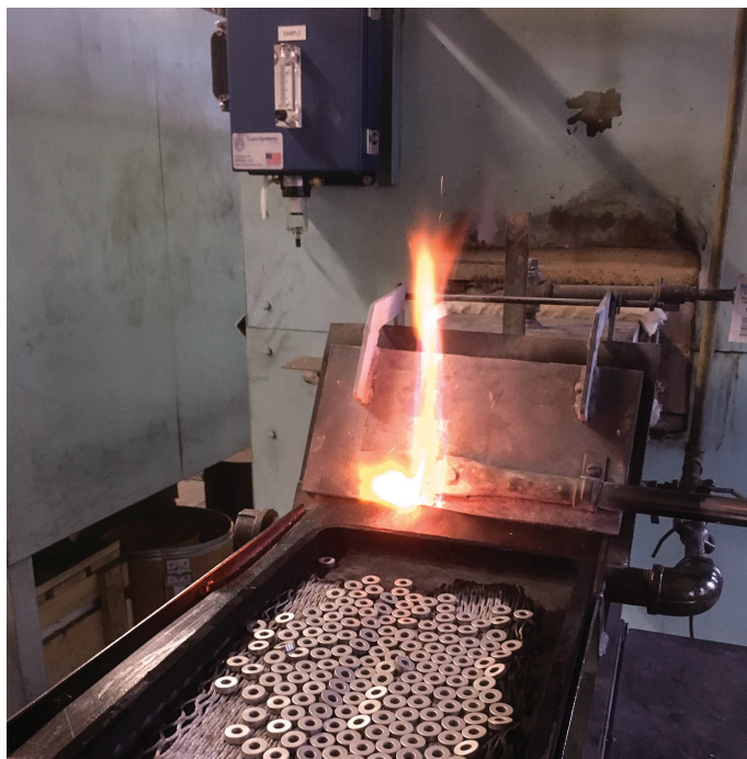
Fig. 2. An atmosphere furnace heat treating parts to adjust their hardness and improve appearance.
