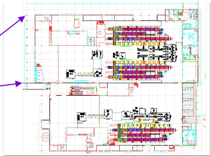
*Possible set-up for 3 production lines at the Herøya facilities, each line with an initial name-plate capacity of 360 MW/year*
